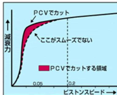
Figure 2. Illustration of PCV Effects (*Courtesy of Öhlins*)
