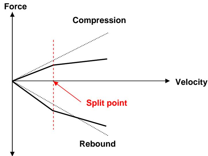
Side note: The damping curve shown above displays an abrupt transition from high to low damping which for some racing applications may not be optimum, as such a sudden transition can upset the dynamics of the car. One advantage with some Öhlins shocks is that they utilize a **PCV (parallel compression valve)** system that allows a smoother damping transition around the split point as shown by the figure below:
