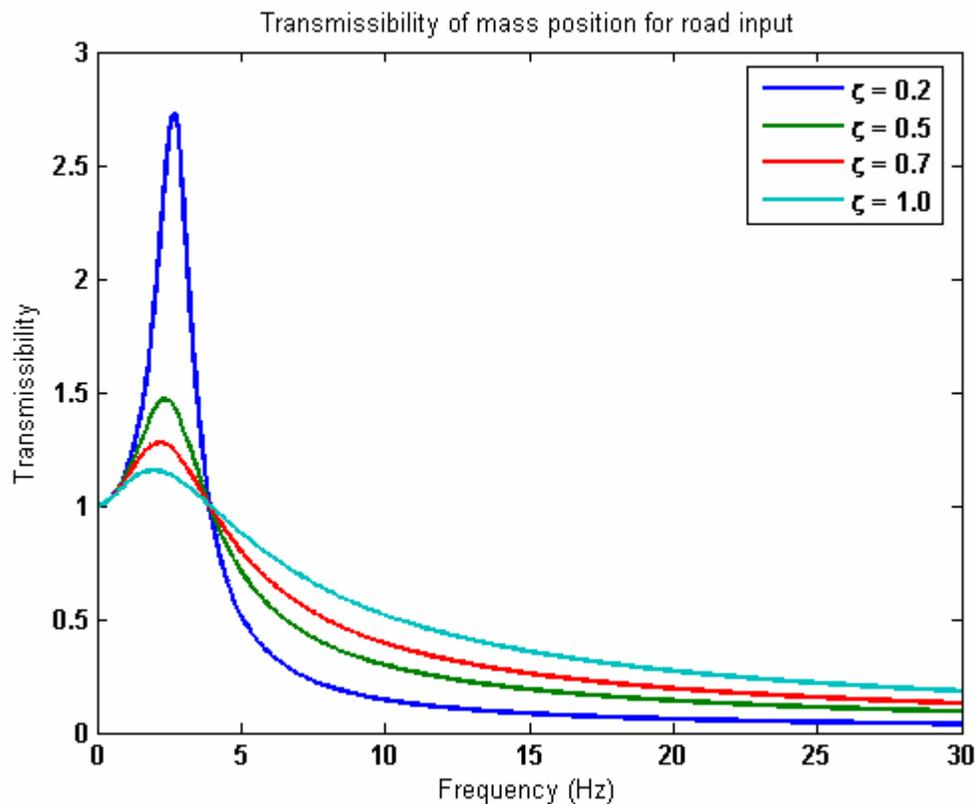
**Figure 1. Transmissibility for different damping ratios**
